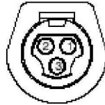
Figure 10. Hypertronics power receptacle, as viewed from the back panel of the NL337. Supply +24V DC on Pin 1. Pin 2 is the supply return and pin 3 is the case ground.
